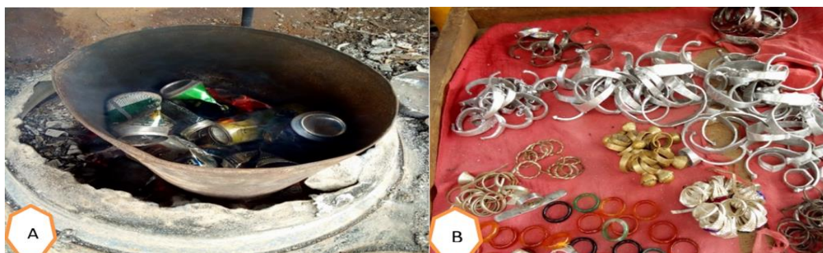
Fig.5: Device for melting beverage cans (A) and jewelry made from recycled objects (B)
