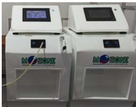
Figure 1 : A pair of Medical Ozone Generator with touchscreen turned on, and ozone output from through silicon hose
