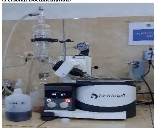
Figure 3. Evaporated Filtrate with Rotary Evaporator (Personal Documentation)
