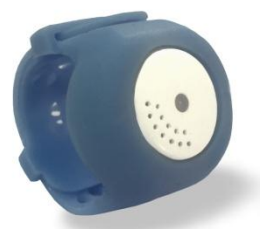
Figure 1: The Bempu Hypothermia Alert Device (TempWatch)
